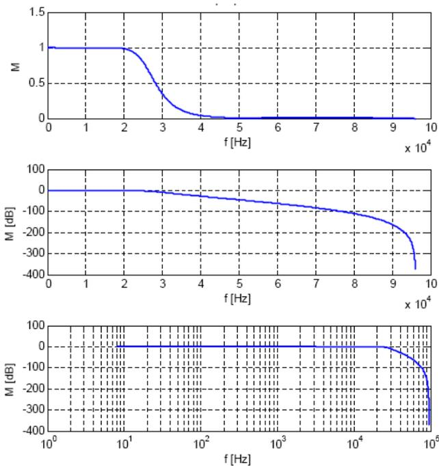
Fig. 4. Frequency characteristic of proposed filter.
