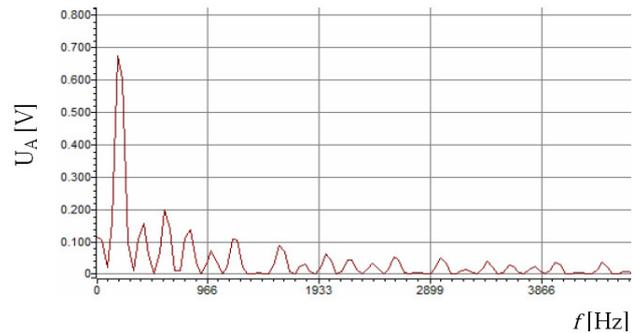
Fig. 13. Amplitude spectrum of square waveform.
