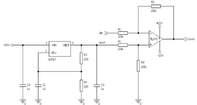
Fig. 3. Block scheme of circuit for voltage adjustment.
