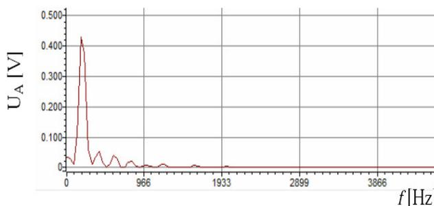
Fig. 11. Amplitude spectrum of triangular waveform.
