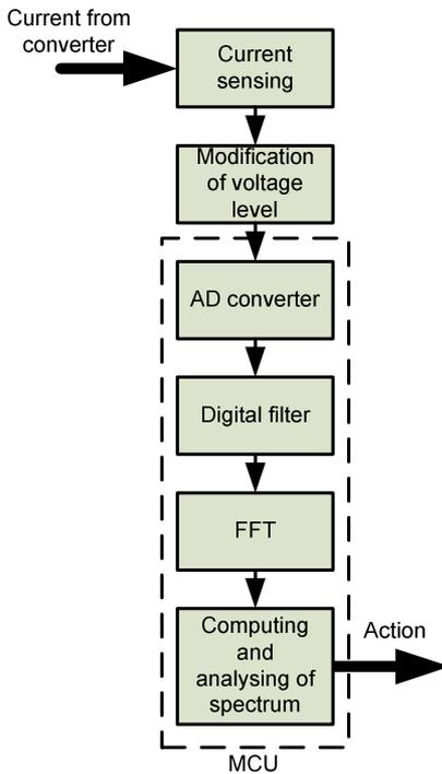
Fig. 1. Block scheme of system for analysis of recuperative currents.
