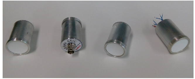
Fig. 3. Picture of the 250 kHz single element air coupled transducers (three transducers on the left) with BNC connector and the 8 elements 400 kHz sectorized array transducer (right) without any connector.
