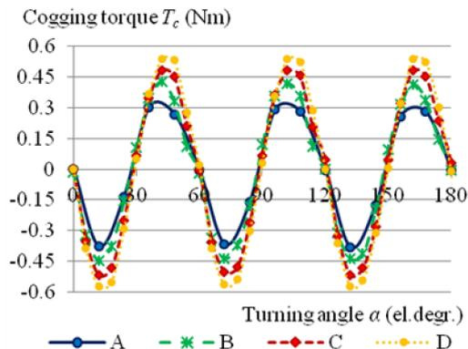
Fig. 8. Curves of cogging torque for different coefficients  $\beta$  ( $n = 4$ ).
