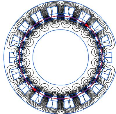
Fig. 4. Modelled magnetic field in PMSG cross section ( $Z_1 = 18$ ,  $2p = 20$ ).
