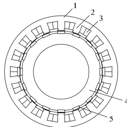
Fig. 2. PMSG in cross section ( $Z_1 = 18$ ,  $2p = 16$ ).
