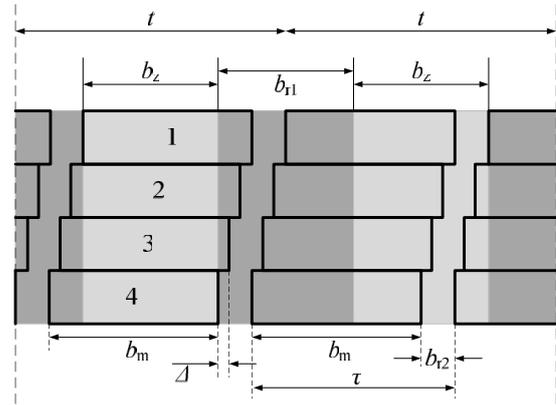
Fig. 6. Principal placement of rotor permanent magnets in axial length  $l$  according to stator teeth (for 2 stator poles  $t$ ).
