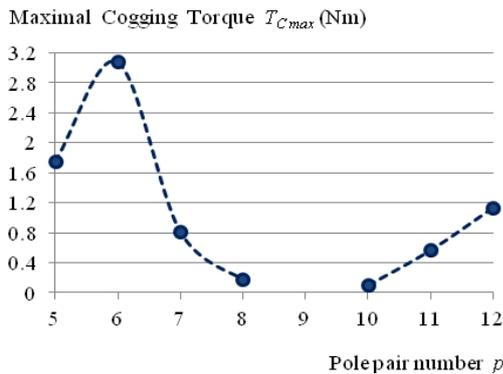
Fig. 5. Maximal values of cogging torque  $T_C$  for PMSG with  $Z_1 = 18$  at different pole pair numbers  $p$  (slot design – opened).
