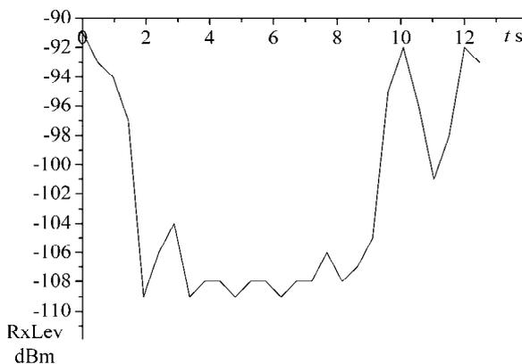
Fig. 2: Received signal level as function of time (MS is moving)
