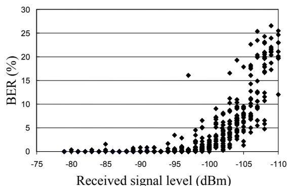
Fig. 3. BER as a function of received signal level
